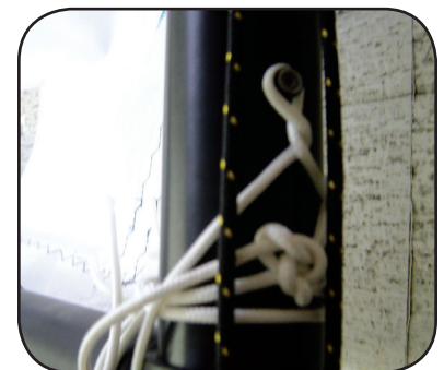
Tightening the preventer for light air - two twists
