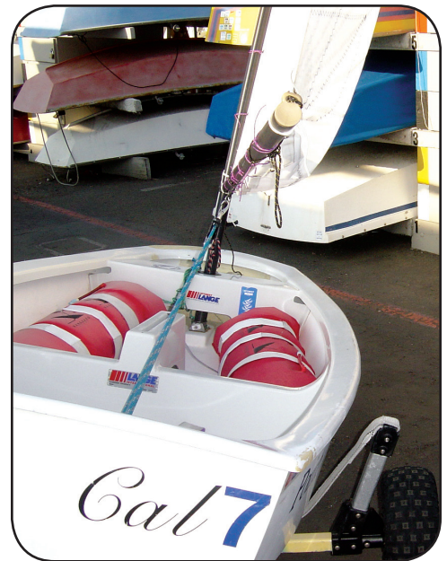
Boom should align with the corner of the boat
